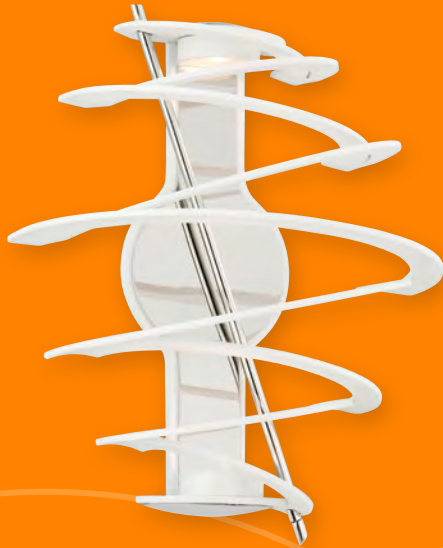
174-11 White LED Sconce W 12" H 14" EXT 6" mm: W 305 H 356 EXT 152 6 / 1.2W LED / 120v (8.5 watt total consumption) 120-277 non-dimming (174-11-I)
